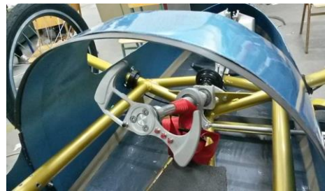
Fig. 10. The trireme vehicle (a) the improved parts designed by a CAD station (b), real parts of the ensemble (c), (d) and details of the steering mechanism (e)
